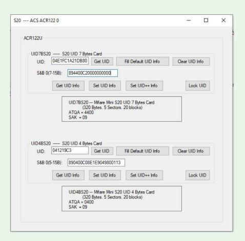
Press the "Set UID Info" button above (the one below would be for S20 cards with a 4-byte UID), the acr122u will beep, a small window will appear saying "SET UID Info Success" and press accept. We can now close the PCSC\_Mifare application.
